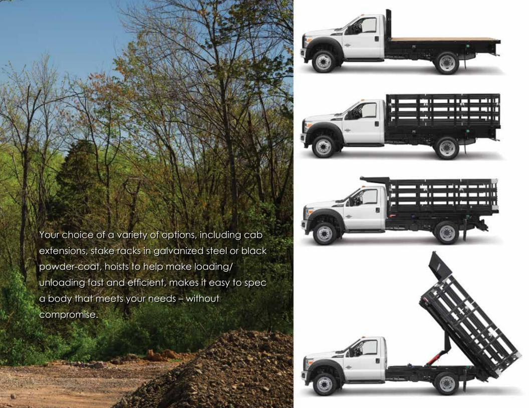
A heavy-duty steel cab extension helps to protect the cab against damage caused by dirt, debris or movement of bulk materials during loading and unloading.
