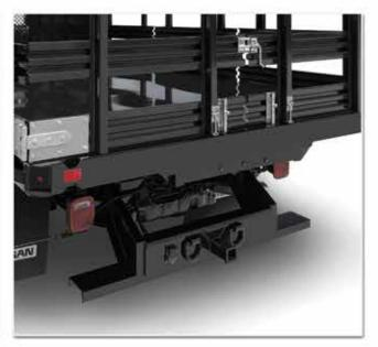
Pre-engineered 2" receiver tube design, the use of ready-to-use molded harness and sealed plug-to-gether connectors, and "universal design" features, such as standard LED body clearance and ID lighting, makes it easy to spec or replace components quickly and efficiently.
