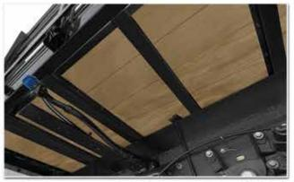
Three-inch I-beam frame construction delivers superior strength and durability. Positioning crossmembers 16 inches on-center reduces weight for better fuel efficiency.
